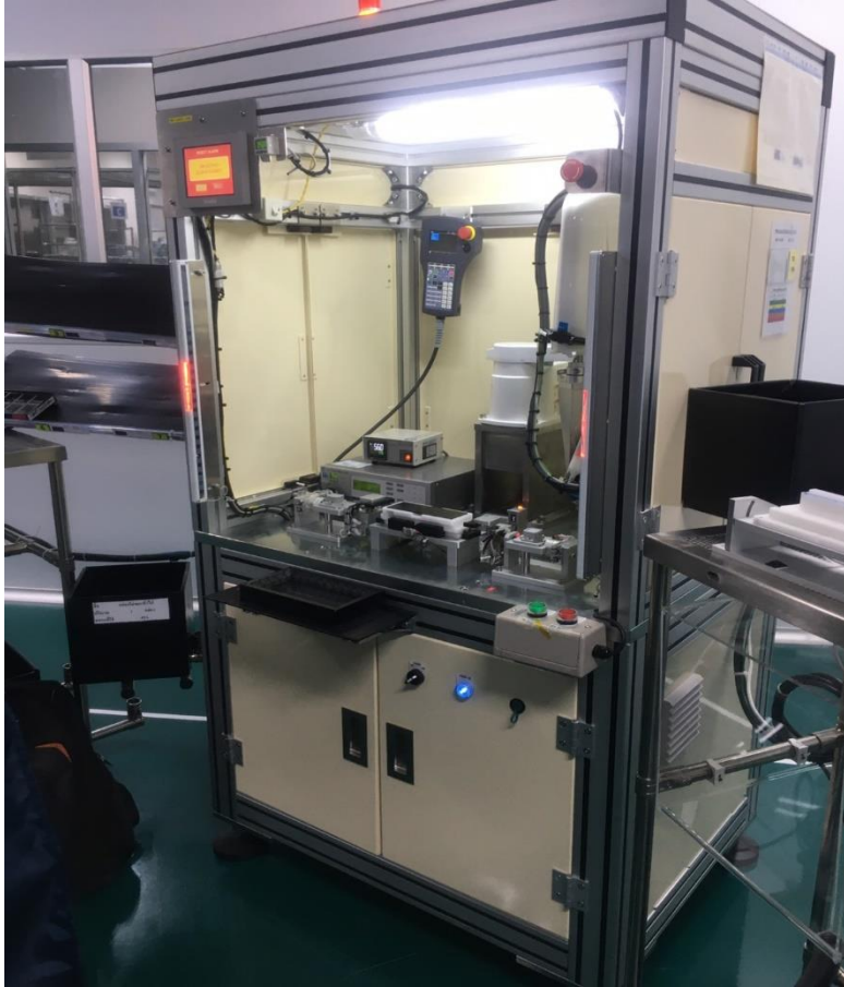
Auto Grease apply with Robotic arm
